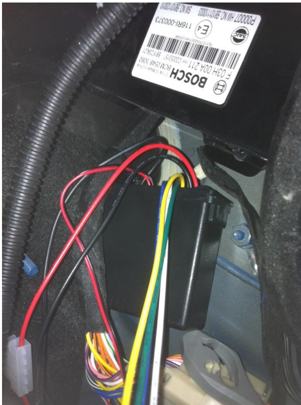
Remove rubber door seal and kick panel , attach control module to inside of panel feed power wire across underneath Intrument panel and go thru the firewall to the battery
