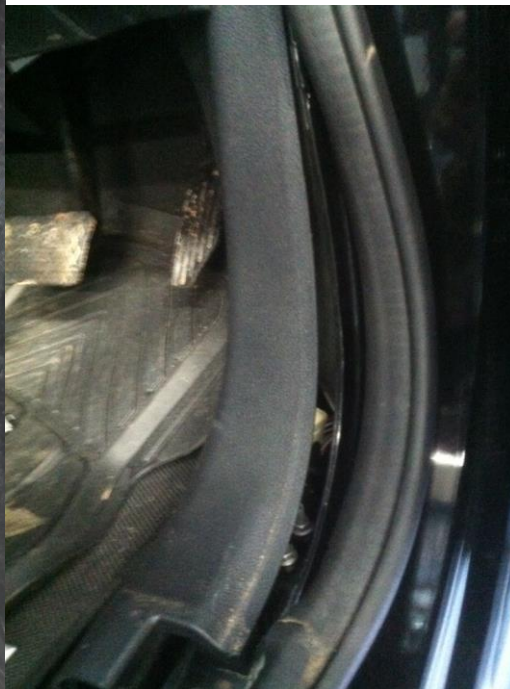
Remove rubber door seal and kick panel , attach control module to inside of panel feed power wire across underneath Intrument panel and go thru the firewall to the battery
