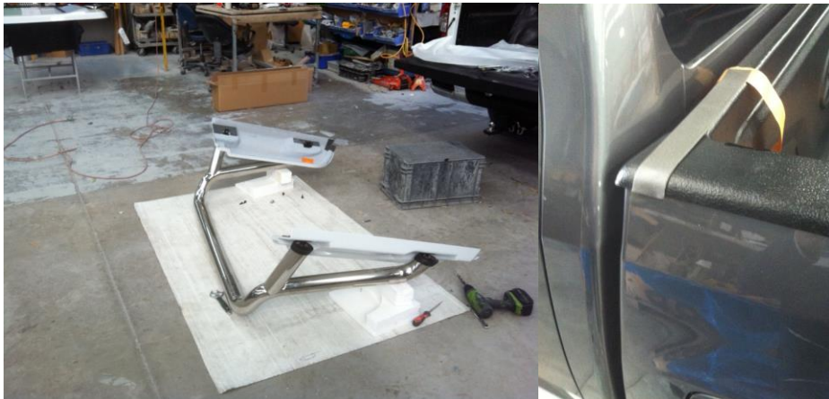
Install foam seal up front across tubliner
