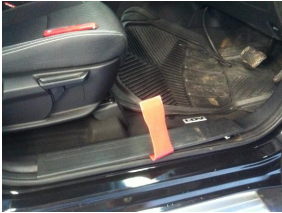
Come up attach grommet and under sil cover –follow harness to kick panel
