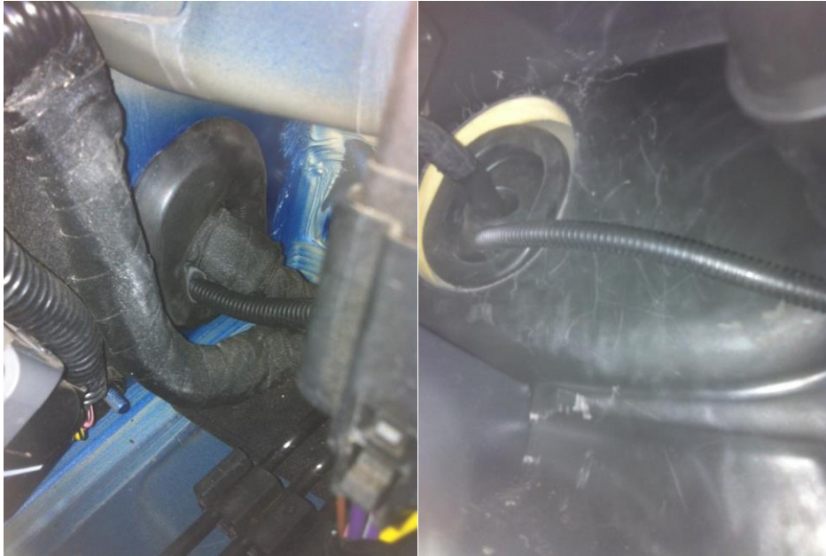
Pierce grommet and feed wire thru fire wall
