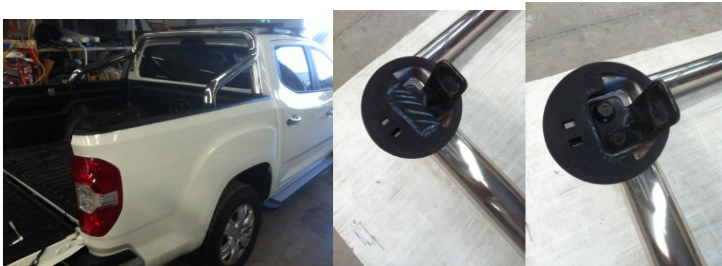
Remove sports bars and place on cushioned surface
