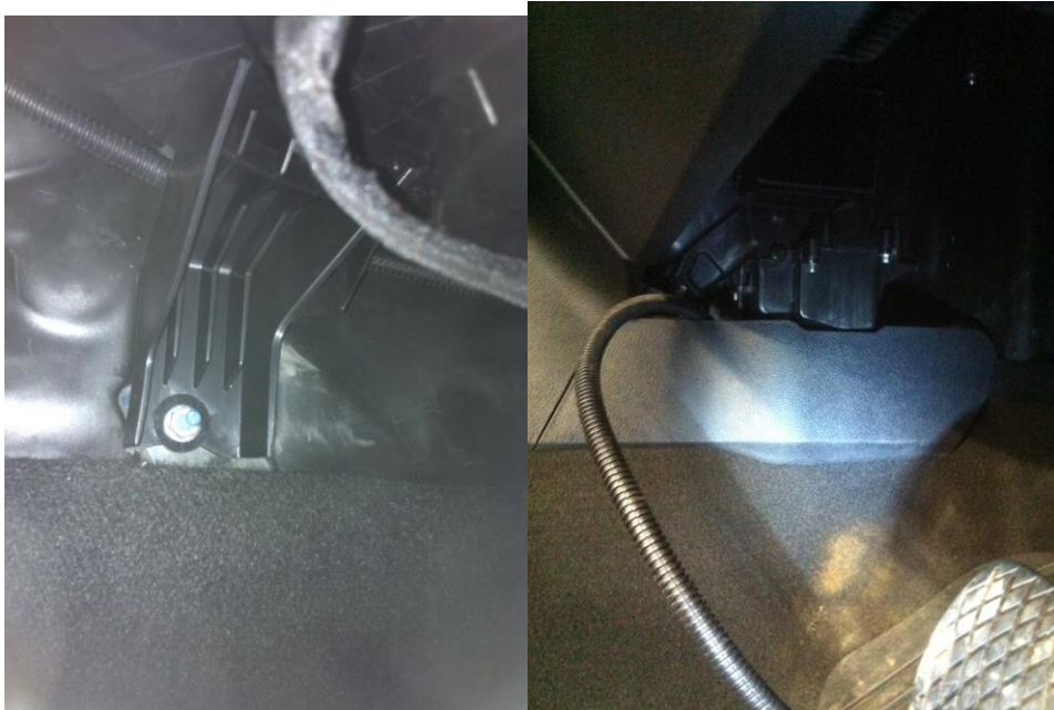
Use conduit on wire anywhere under the bonnet , use cable ties to secure.
